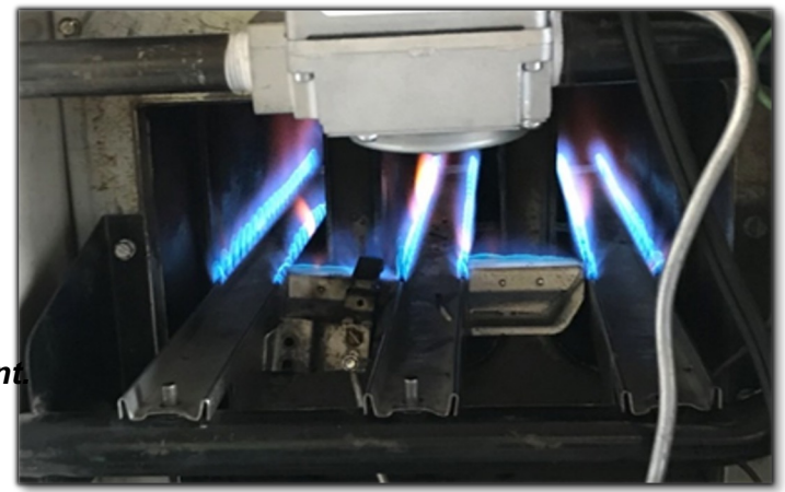
Visual flashback and flame characterization testing.
